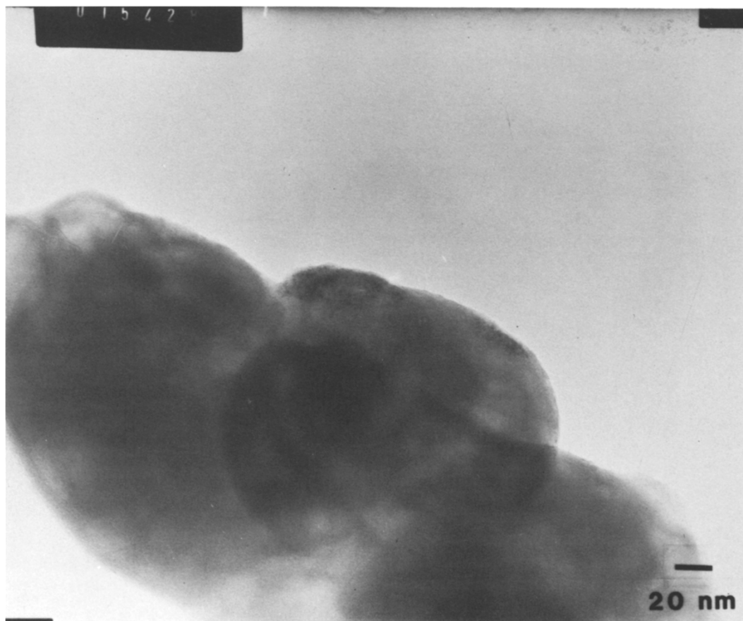
FIG. 2. TEM micrograph of RuCaA[SD].
